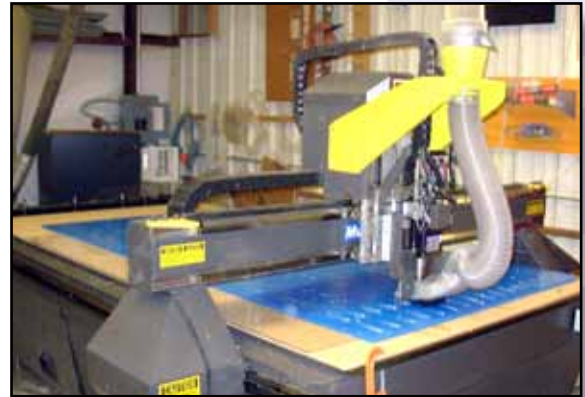
The MultiCam Router cuts slots for JC Penney kids' shoe displays.
