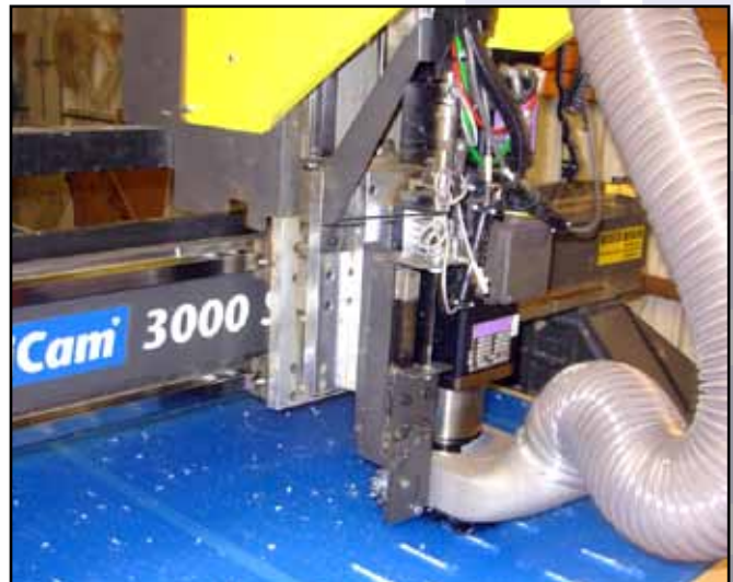
Plex-Appeal's MultiCam Router features a 5.5-hp, 32,000-rpm spindle with automatic tool changer.
