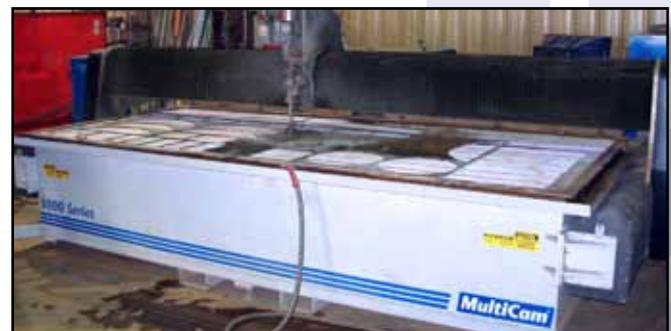
*NTPV’s MultiCam 3000 Series WaterJet features a 60" x 144" work surface.*
