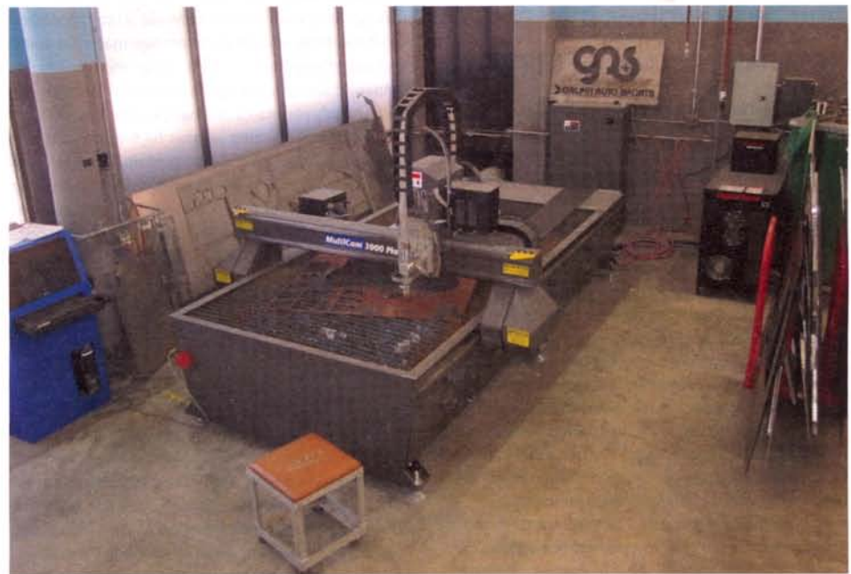
Figure 4 The customization shop at Galpin Auto Sports now includes a plasma cutting table as well as several hand-held plasma cutting systems.
