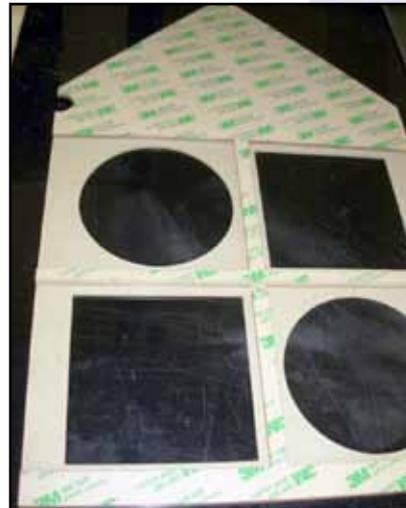
The laser cuts multiple adhesive-backed pieces and inserts to combine into stick-and-peel signs.
