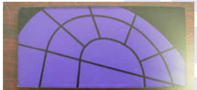
Laser scoring of the paper backing allows creative painting techniques.
