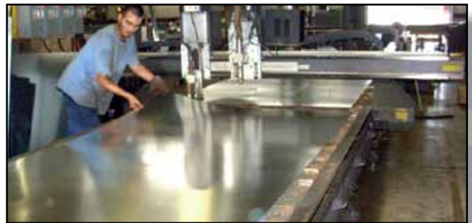
A pendulum processing feature lets the MultiCam Plasma cut one sheet while the operator loads another.
